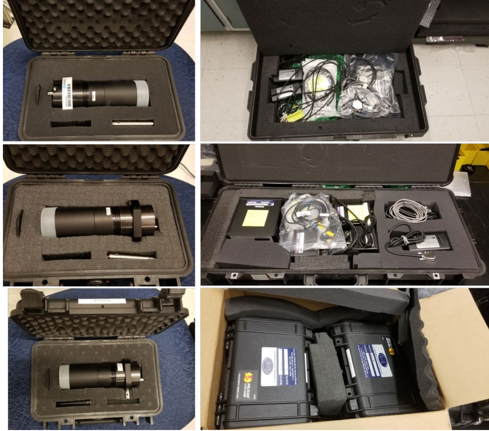
Figure 1.1 Photographs of NASA IGA DET-8 radiometers (Numbers 106, 107, and 109) as received. The radiometers were packaged in individual pelican cases (left) and combined in boxes with ancillary equipment consisting of the L-1 temperature controllers and transimpedance amplifiers. A new amplifier for DET-8-106 was received later, directly from the manufacturer.
