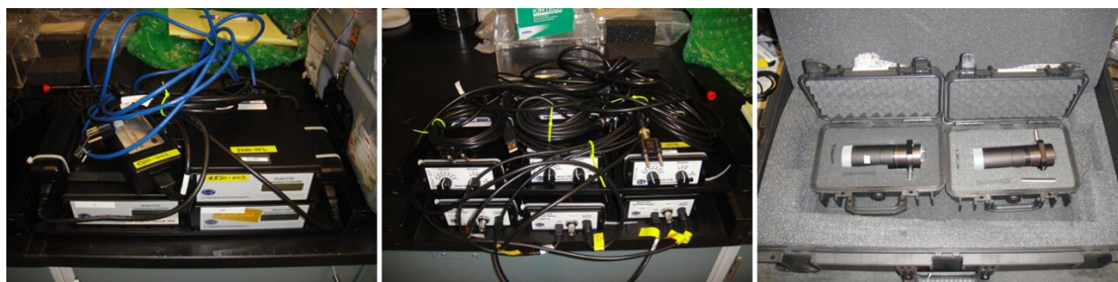
Figure 1.1 Photographs of GLAMR Si Radiometer as received consisting of the L-1 temperature controller (left), transimpedance amplifier (middle), and radiometer (right). The temperature controller and transimpedance amplifier were received together with the same components for the IGA and exIGA radiometers whereas the Si radiometer was packaged with the IGA radiometer.
