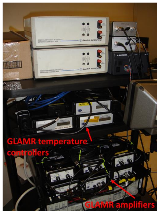
Figure 2.3 Photograph showing the setup of the GLAMR temperature controllers and transimpedance amplifiers
