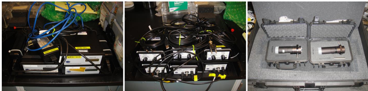
Figure 1.1 Photographs of GLAMR IGA Radiometer as received consisting of the L-1 temperature controller (left), transimpedance amplifier (middle), and radiometer (right). The temperature controller and transimpedance amplifier were received together with the same components for the IGA and exIGA radiometers whereas the IGA radiometer was packaged with the Si radiometer.
