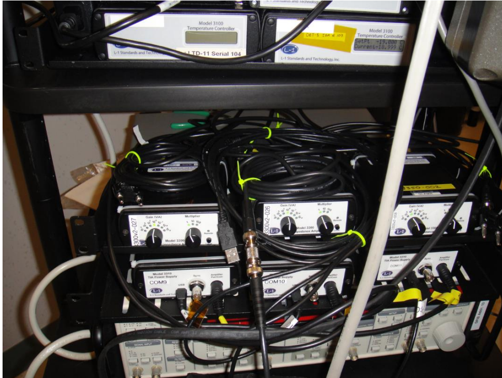
Figure 2.3 Photograph showing the setup of the GLAMR temperature controller and transimpedance amplifiers
