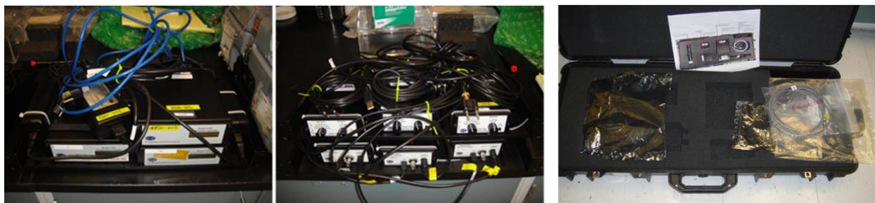
Figure 1.1 Photographs of the GLAMR ex-IGA detector as received. The temperature controller (left) and transimpedance amplifier (middle) were received with the same devices associated with the silicon and IGA radiometers. The GLAMR ex-IGA radiance meter was received packaged in a pelican case (right).
