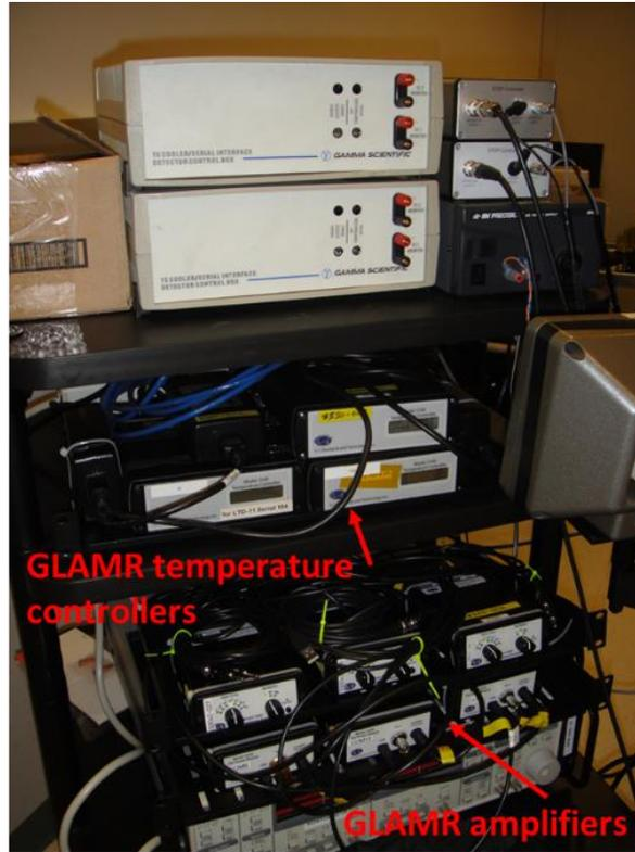
Figure 2.2 Photographs showing the control box setup for GLAMR including the transimpedance amplifiers and temperature controllers and the step controller for SIRCUS Pyro #1
