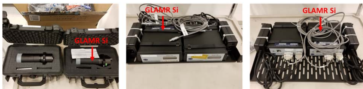
Figure 1.1 Picture of GLAMR Si Radiometer as received, where it was packaged together with the GLAMR InGaAs Radiometer. The leftmost picture shows the radiometer and the box containing the transimpedance amplifier. Front (middle) and back (right) views of the temperature controller are also shown.
