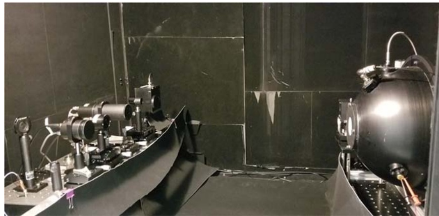
Figure 2.2 Side-view of detector bench setup for radiance measurements of the DUT using both T-01 and IRD WS #2 as the standard reference detectors.
