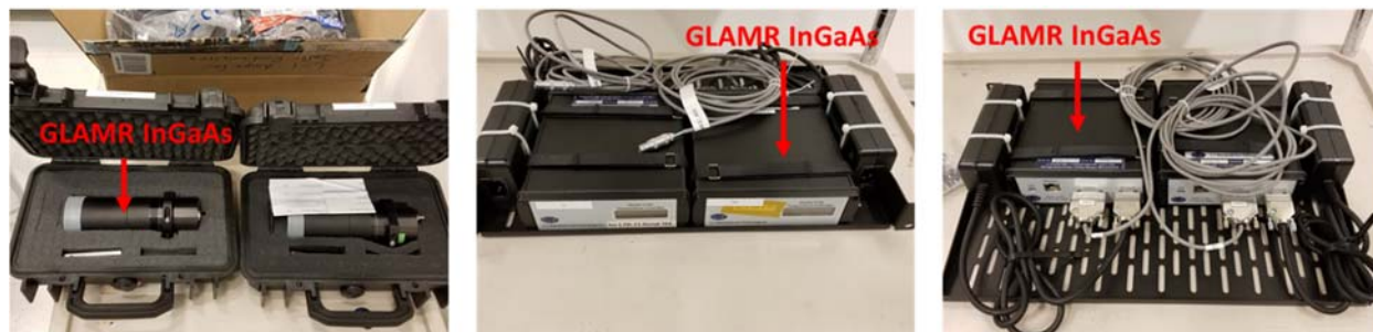
Figure 1.1 Picture of GLAMR IGA Radiometer as received, where it was packaged together with the GLAMR Si Radiometer. The leftmost picture shows the radiometer and the box containing the transimpedance amplifier. Front (center) and back (right) views of the temperature controller are also shown.
